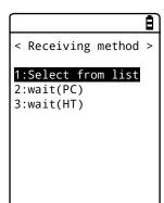
Select "Select from list" to get the file list from the sending side. The receiving side can select the files to be received from the list. > Step [2] Select "2:Wait (PC)"/"3:Wait (HT)" to enter the reception wait state immediately. If the sending side is a PC, select "2:Wait (PC)"; if it is GTX-221-G, select "3: Wait (HT)". Files to be received depend on the sending side. > Step [3]
