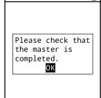
Completion of Clone cannot be confirmed on the copy terminal. Be sure to confirm on the screen on the master terminal that the transfer operation has been completed. If you find on the master terminal that the transfer operation has not been completed, execute Clone again.
