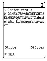
The scanned barcode, barcode type and number of bytes will be displayed.
