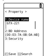
While [F1] or [F2] is displayed at the bottom of the screen, press the corresponding key to display its submenu or to execute its function (special feature).
